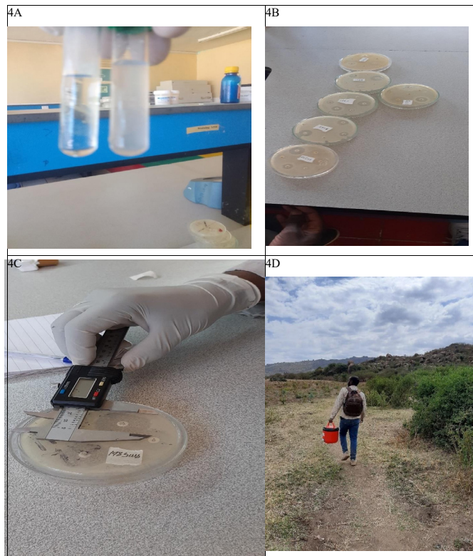
Supplementary Figure 4: A= McFarland turbidity, B= Antimicrobial sensitivity test, C= measurement of inhibition zone by digital caliper, D= .....?.
