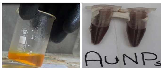
Figure 1: Color changes were observed: from yellow-brown to dark brown for silver nanoparticles (AgNPs) and from pink to reddish-brown or yellowish for gold nanoparticles.
