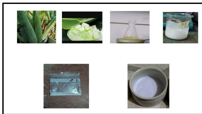
Figure 1: Green synthesis of zinc oxide nanoparticles. Fresh Aloe vera leaves were collected. The leaves were washed and cut for preparing the extract. The extract was added to the zinc acetate solution. NaOH was slowly added to the mixture until the color of the mixture turned from clear bright yellow to a little turbid and a white precipitate began to form. White ZnO NPs were totally precipitated. White powder of ZnO NPs was obtained after calcination at 400 °C.
