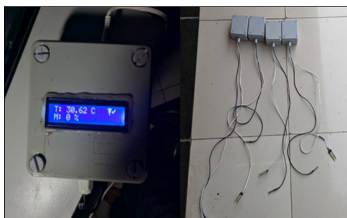
Figure 7: LCD Visualize real-time data for temperature and moisture and replication of the prototype
