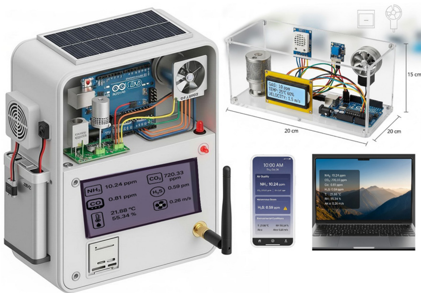
Figure 1: System for measuring gas, temperature, humidity, and air speed
