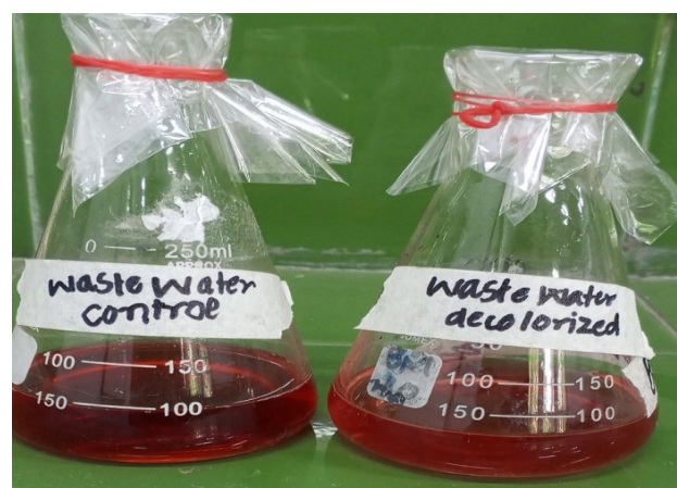
Fig. 3. Flask 1, containing only wastewater, acts as a control, whereas flask 2 contains decolorized wastewater treated with the fungal strain.
