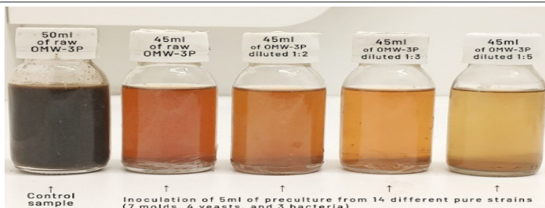
Figure 5: Decolorization of OMW-3P after 15 days of treatment with a consortium of 14 purified strains (7 molds, 4 yeasts, and 3 bacteria)
