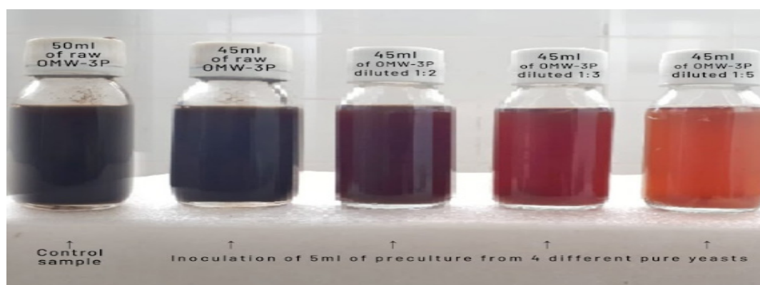
Figure 3: Decolorization of OMW-3P after 15 days of treatment with a mixed culture of 4 purified yeast strains
