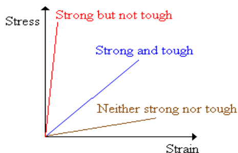
Figure 13.5 graphical representation of toughness and strength
